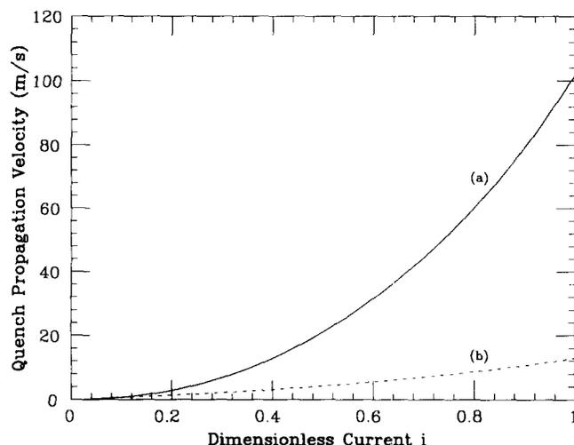
Figure 2 Quench propagation velocity as a function of dimensionless current,  $i$ : (a) taking into account current redistribution; (b) assuming instantaneous current redistribution
