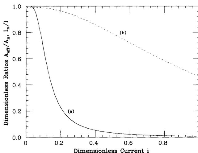
Figure 3 Dimensionless ratios characterizing the effectiveness of the stabilizer as a function of dimensionless current,  $i$ : (a) effective stabilizer area normalized to total stabilizer area,  $A_{\text{eff}}/A_n$ ; (b) current in stabilizer normalized to total transport current,  $I_n/I$
