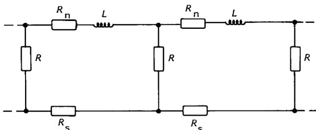
Figure 1 Effective electrical circuit describing the current distribution in the conductor
