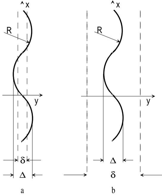
Fig. 1. Trajectory of electron motion near the domain wall: a)  $\Delta \gg \delta$ , b)  $\Delta \ll \delta$ .
