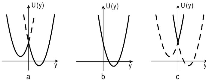
Fig. 2. The field  $U(y)$  is represented by the solid line. Depending on the sign of  $d$ , it consists of different parts of two identical parabolic potential wells: a)  $d < 0$ , b)  $d = 0$ , c)  $d > 0$ .
