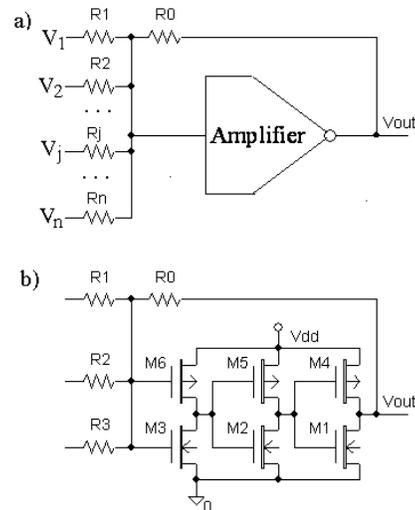
**Figure 1.** Summing amplifier: a) general structure; b) CMOS implementation example.
