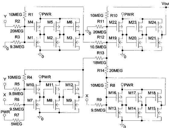
Figure 8. CMOS implementation of fuzzy controller for washing machine.
