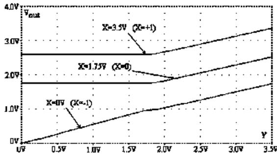
Figure 9. Results of SPICE simulation for controller on the Fig.8.
