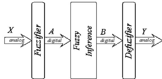
**Figure 5.** Fuzzy device structure.
