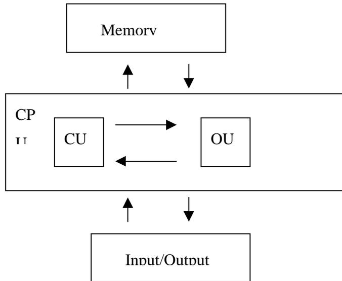
Figure 1: Digital computer structure
