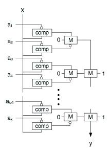
Figure 2. Comparator array structure
