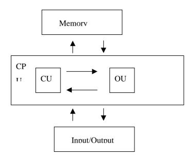
Figure 1: Digital computer structure
