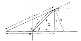
x: abscissa, y: ordinate, s: arclength, r: radius, a: polar arc,  $\sigma$ : subtangent,  $\tau$ : tangent, v: normal,  $Q = \widehat{OPR}$ : area between curve and X-axis, xy: circumscribed rectangle
