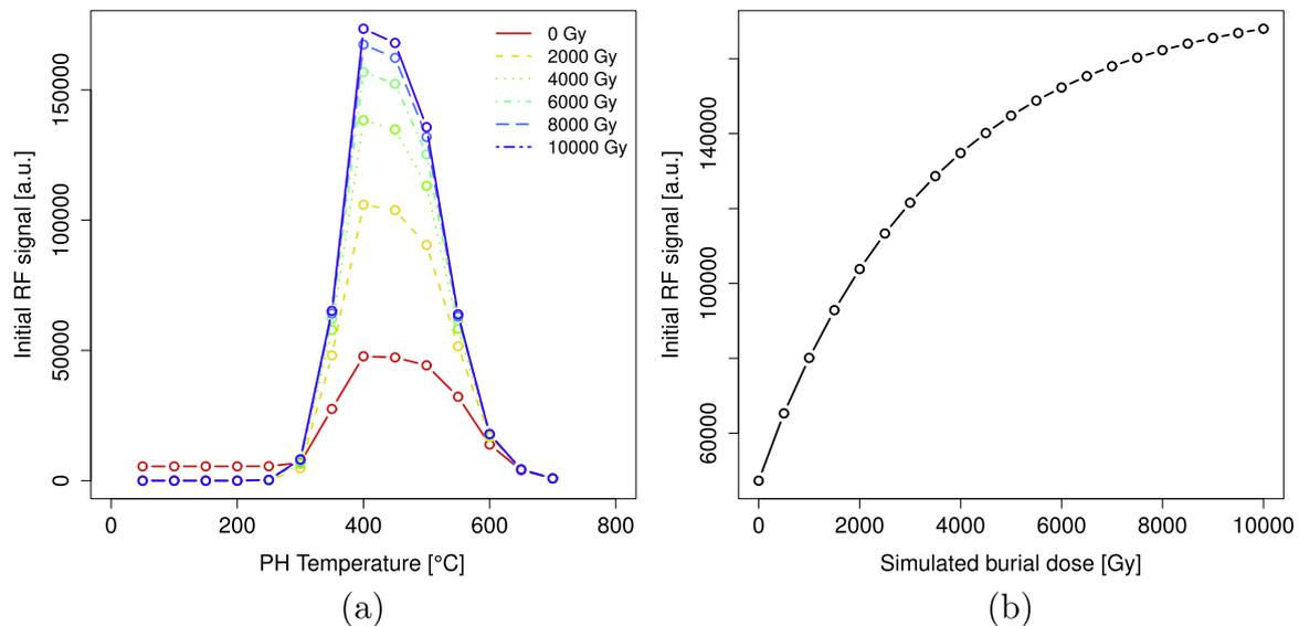
**Fig. 10.** Simulations for different burial doses for step 7 in the sample history (see step 7 in Table 3). (a) shows initial RF signals for different preheat temperatures and for 6 different burial doses. (b) is a detailed view on the initial RF signal at 450 °C. The initial signal was plotted against the simulated burial dose.
