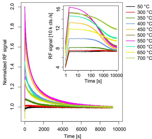
**Fig. 2.** UV-RF signal for sample BT1195 for different preheat temperatures (holding for 120 s). The values are normalized to the last data point of each measurement. The total absorbed dose was 600 Gy during each RF measurement. For the sake of clarity the UV-RF curves for preheat temperatures from 100 °C to 250 °C were removed, because no change was observed. The inset shows the same data as the main figure but with absolute values and a logarithmic x-axis.
