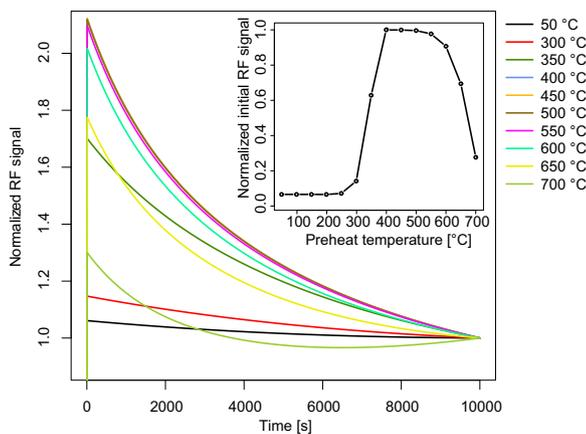
**Fig. 6.** Simulation of the sequence presented in Table 3 with the parameters from Table 2. The RF signal is normalized to the last signal value at 10,000 s. The inset shows the simulated initial RF signal from the main figure. The values on the y-axis are normalized to the highest value of all initial signals.
