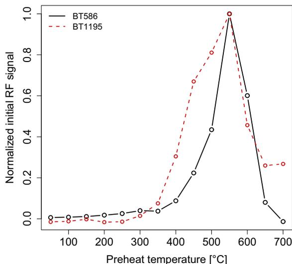
**Fig. 3.** Initial UV-RF signal for different preheat temperatures (holding for 120 s) for samples BT586 and BT1195 normalized to the initial signal at 550 °C.
