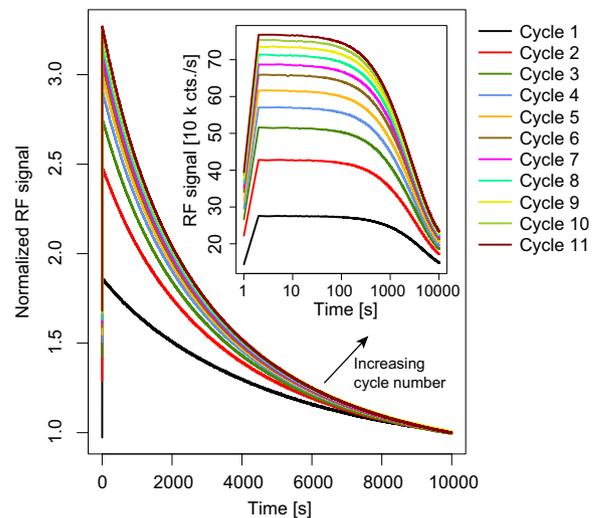
**Fig. 4.** UV-RF signals for sample BT586 for 11 cycles for a preheat at 500 °C for 120 s between each cycle. The total absorbed dose was 600 Gy for each RF cycle. The curves are normalized to the last data point. The inset shows the same data as the main figure but with absolute values and a logarithmic x-axis.
