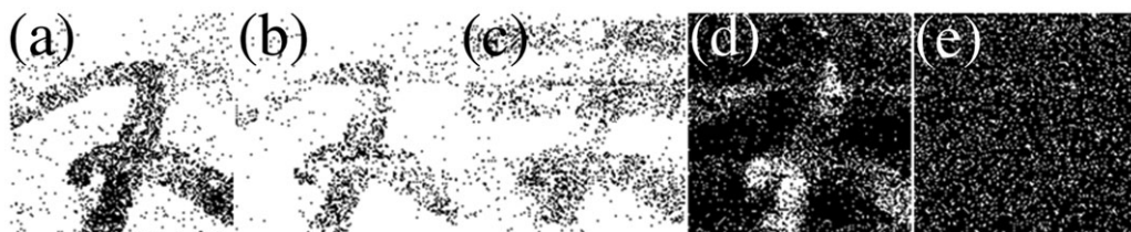
Figure 3 Examples of different I_{\lambda} images, with black pixels indicating 'signal'; that is, a peak found by our methodology. (a) \sim 1460\text{ cm}^{-1} , an 'ink' signal; (b) \sim 1860\text{ cm}^{-1} , an 'ink' signal; (c) \sim 1580\text{ cm}^{-1} , an 'ink' signal; (d) \sim 1120\text{ cm}^{-1} , a 'clay' signal; (e) \sim 3920\text{ cm}^{-1} , typical white noise.
