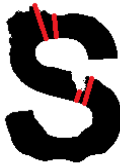
Figure 7.1 Example of local-scale stroke width discontinuity due to stains and letter erosion (discontinuities marked in red ).
