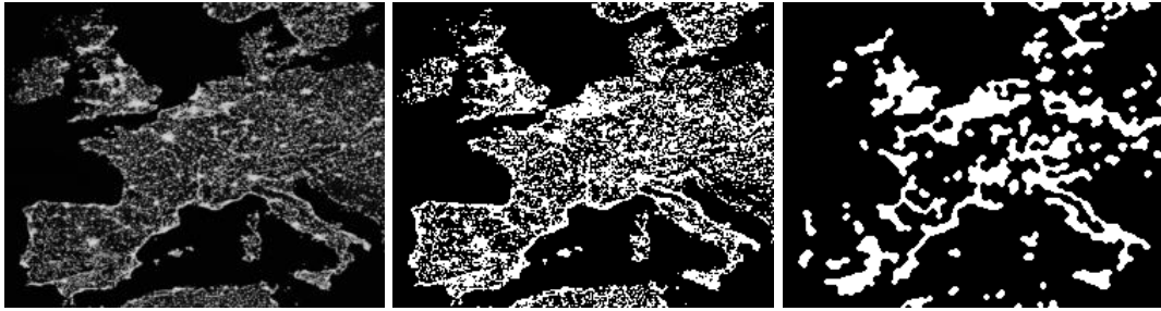
Figure 10.3 Segmentation of a satellite image of Europe night-lights: original image ( left ), vs. Otsu binarization ( center ), vs. result with the default setting ( right ). Image courtesy NASA/Goddard Space Flight Center Scientific Visualization Studio, public domain.
