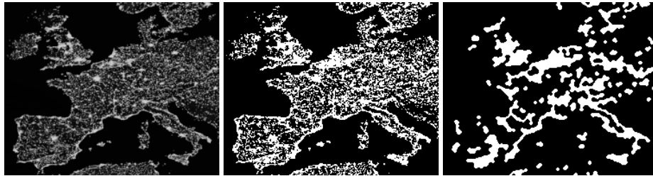
Fig. 3. Segmentation of a satellite image of Europe night-lights: original image ( left ), vs. Otsu binarization ( center ), vs. result with the default setting ( right ). Image courtesy NASA/Goddard Space Flight Center Scientific Visualization Studio, public domain
