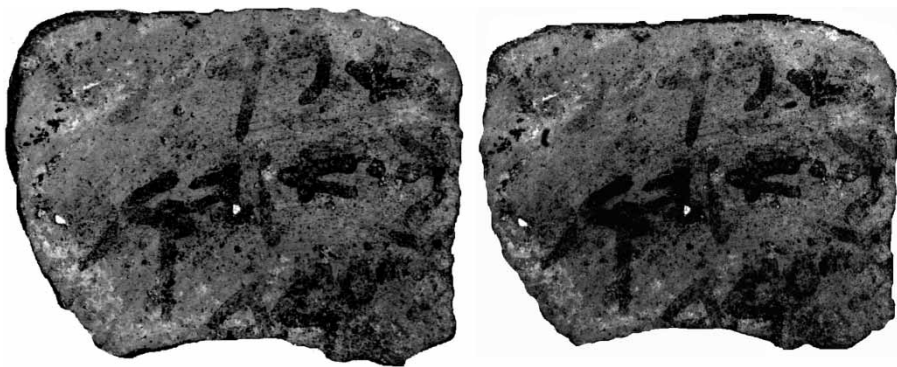
Fig. 11. Images of Inscription No. 1 from Ḥorvat Radum. Left, image photographed using the low-cost system at wavelength 635 nm; right, image photographed with a high-cost commercial multispectral imager at wavelength 635 nm.
