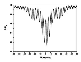
FIG. 2. Typical magnetoresistance plot as measured in a sample with a layer of  $8000\ \text{Å}$  Cu.
