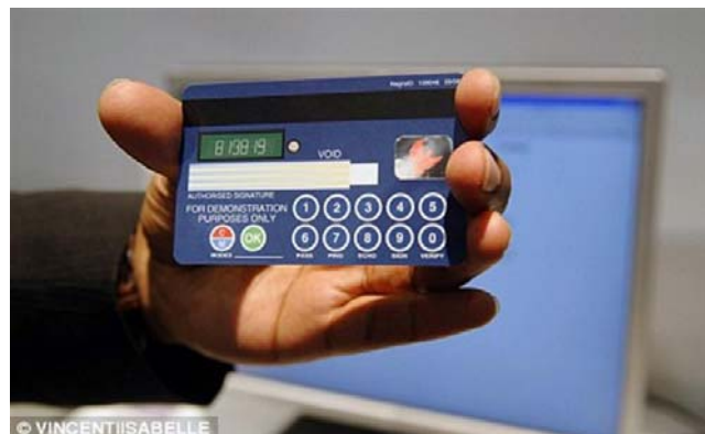
Figure 4. | Smart credit card with a flat battery one millimeter thick. Courtesy of EMUE Co.
