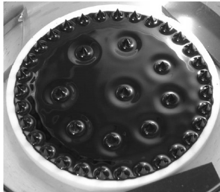
Fig. 10. Nine 'solitons' (solitary structures), each generated by a transient, local pulse of magnetic field applied in the subcritical range 1-2 of Fig. 8. Peaks along rim of the container are an artifact due to the curved surface of the meniscus. The containing vessel is 12 cm in diameter and the liquid depth is 3 mm. Adapted from Ref. 41.
