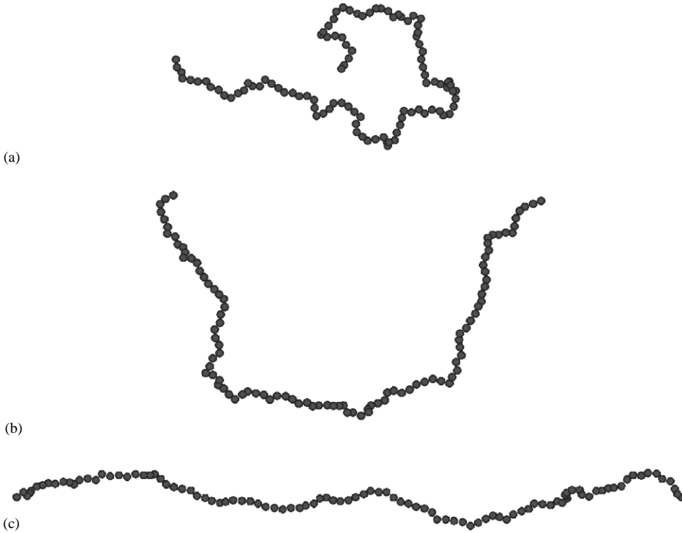
Fig. 6. Snapshots of Monte-Carlo simulations of a PE chain consisting of N=100 monomers of size b . In all simulations, the bare persistence length is fixed at \ell_0/b = 1 , and the charge-interaction parameter is chosen to be \tau^2 \ell_B \ell_0 = 2 . The snapshots correspond to varying screening length of: (a) \kappa^{-1}/b = \sqrt{2} , leading to an electrostatic contribution to the persistence length of \ell_{\text{OSF}}/b = 1 , (b) \kappa^{-1}/b = \sqrt{18} , leading to \ell_{\text{OSF}}/b = 9 , and (c) \kappa^{-1}/b = \sqrt{200} , leading to \ell_{\text{OSF}}/b = 100 . According to the simple scaling principle, Eq. (3.10), the effective persistence length in the snapshots (a)–(c) should be similar to the bare persistence length in Fig. 4(a)–(c).
