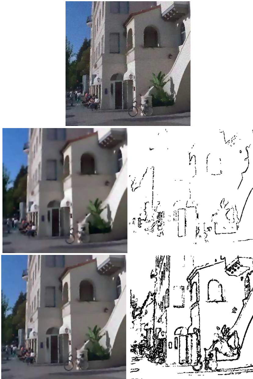
FIG. 4.1. Top: Noisy image. Left: Denoising based on the standard scheme ( \beta = \sqrt{0.0001} middle and \beta = \sqrt{0.002} bottom). Right: Edge detection through the nonnegativity condition ( \beta = \sqrt{0.0001} middle and \beta = \sqrt{0.002} bottom). Parameters: 25 iterations, h = 1/305 , \Delta t = 0.00006 .
