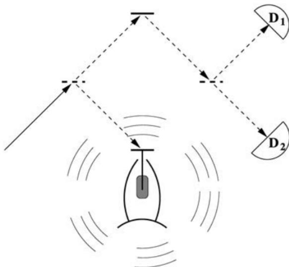
Fig. 7. The Penrose bomb-testing device. The mirror of the good bomb cannot reflect the photon, since the incoming photon causes an explosion. Therefore,  $D_2$  sometimes clicks. The mirror of a dud is connected to the massive body, and therefore the interferometer “works,” i.e.,  $D_2$  never clicks when the mirror is a dud.
