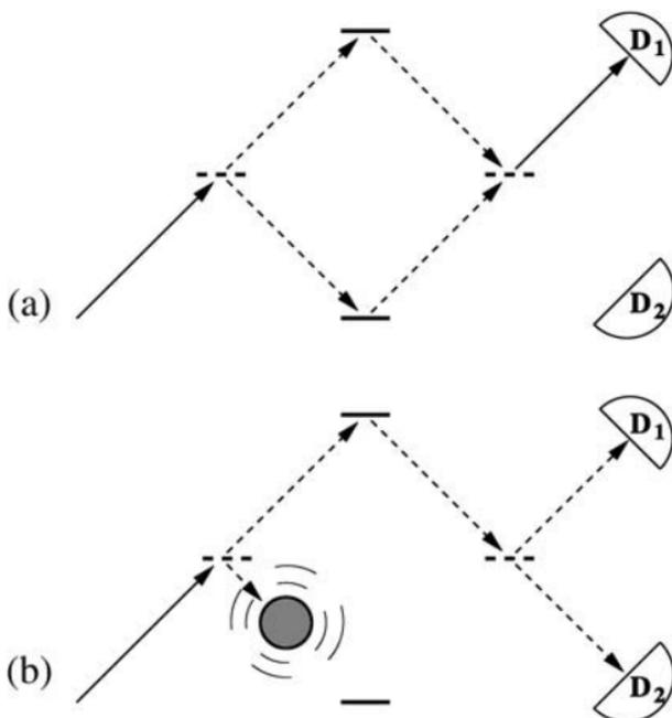
Fig. 1. (a) When the interferometer is properly tuned, all photons are detected by  $D_1$  and none reach  $D_2$ . (b) If the bomb is present, detector  $D_2$  has the probability 25% to detect the photon sent through the interferometer, and in this case we know that the bomb is inside the interferometer without exploding it.
