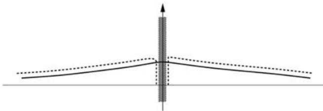
Fig. 4. Dicke's Experiment. The ground state of a particle in the potential well (solid line) is changed to a more energetic state (dashed line) due to a short radiation pulse, while the quantum state of the photons in the pulse remains unchanged.
