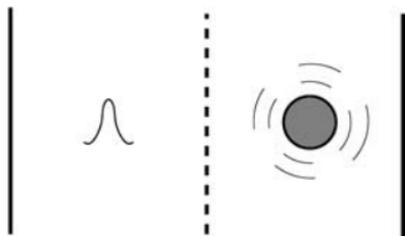
Fig. 8. The almost 100% efficient scheme of the IFM. If there is a “bomb” or a nontransparent object in the right cavity, then the photon stays in the left cavity, with a probability to go to the right cavity which can be made arbitrary small by increasing the reflectivity of the mirror between the cavities. If, however, the right cavity is empty, then after some time the photon will move there with certainty.
